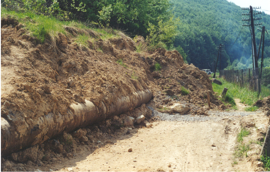
Fig. 19. Failed water pipe-line by landslide in Hriňová village (Middle Slovakia – Photo M. Kopecký)
